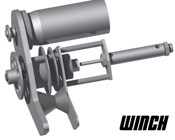
In order to have a linear punch launcher powered simply with surgical tubing, a winch was needed to retract the punch and stretch the tubing. The winch is powered by an off-the-shelf drill transmission which does not backdrive, thereby holding it's position even when unpowered! A simple cylinder disengages a dog gear allowing the winch to free spin and release the punch.
